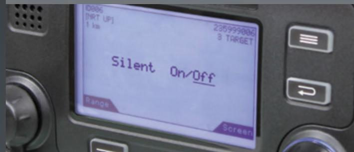
The transmit functionality of the A100 can be switched on and off whilst continuing to receive all AIS messages.
